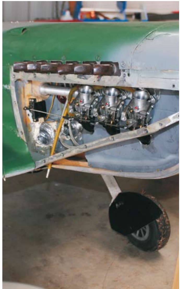
ROTO 135 three cylinder four stroke
