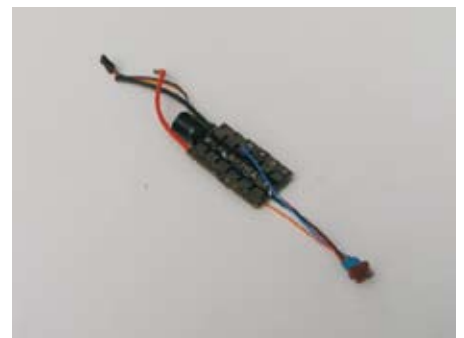
Electric motor speed controller 15 Amp 120 gram.
