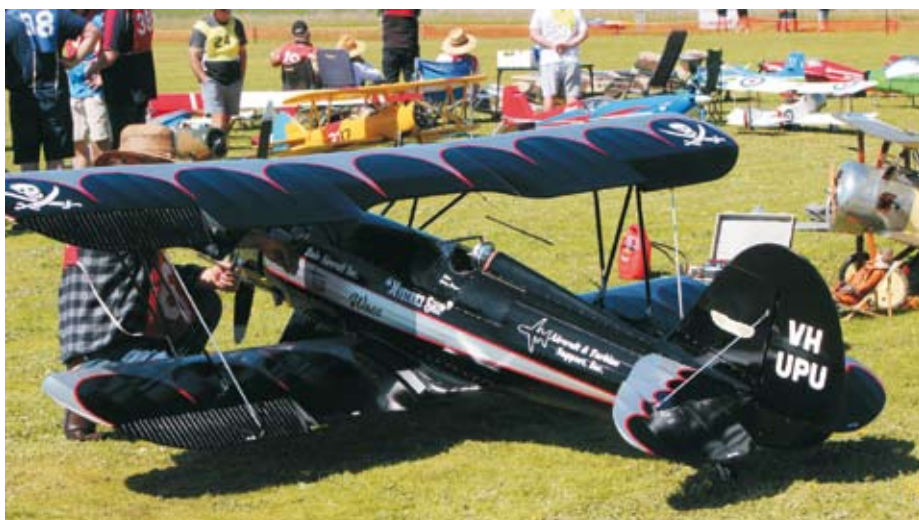
38kg - twin 5,000 mAh battery packs - thirty month build
