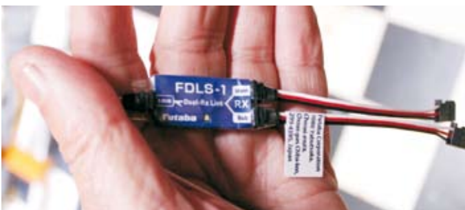
For twin receivers into a power supply
