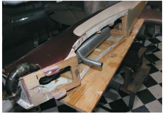
Large internal canister muffler takes up a lot of room
