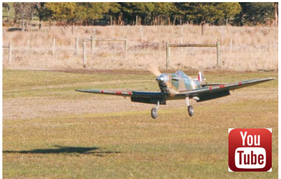
Stable approach with 2mm up elevator mixed and forty five degrees of split flap
