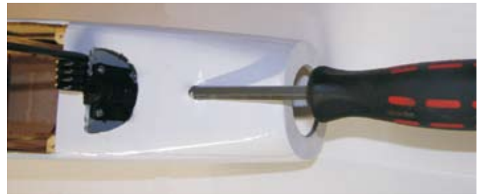
Make your own access to service the nose gear steering arm.
