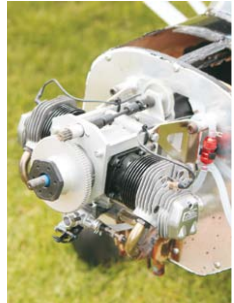
Shuts the OS Super Gemini down and re-starts using this FEMA onboard starter
