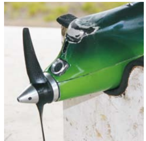
See the venturi? That's a binary throttle, on or off.
