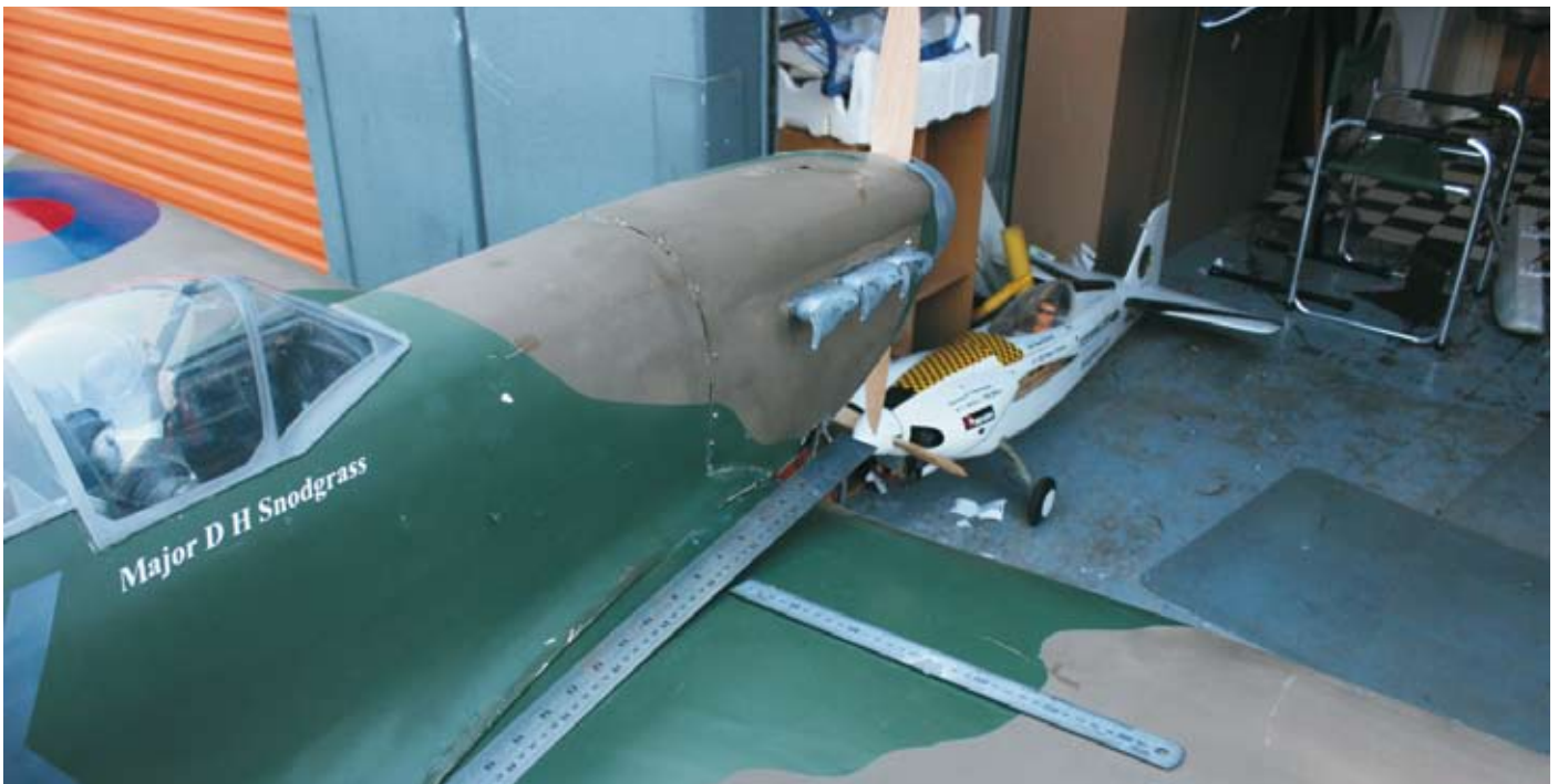
Tank empty gear down the CofG is 195mm from the leading edge. Measured at its widest point up elevator throw set at 35mm produces a good flying experience
