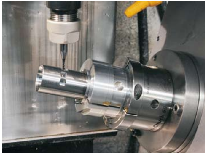
Cutting the inlet ports into the cylinder
