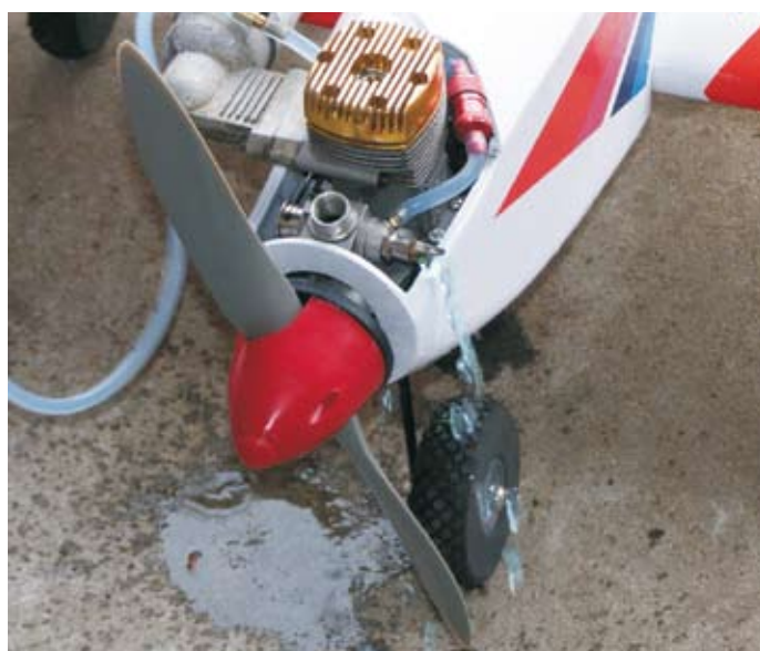
Remove the needle and flush the jet through.
