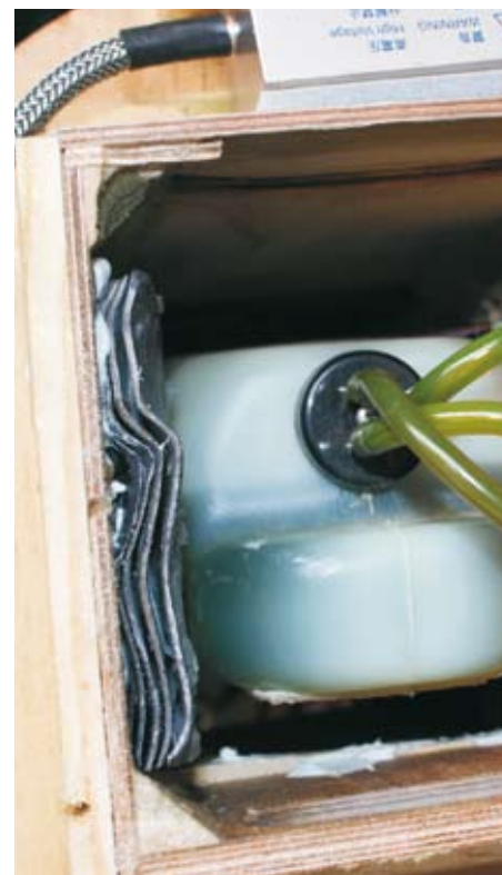
Lead glued with silastic
