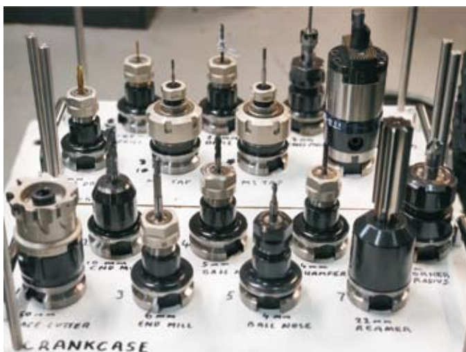
Production tools used to manufacture the crankcase
