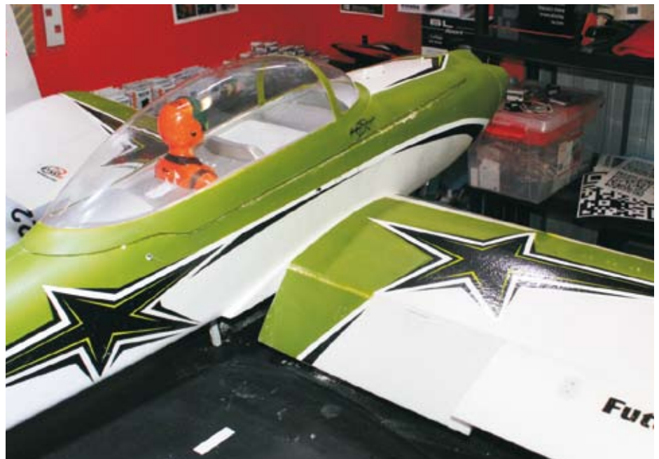
60mm of flap with 3mm of flap elevator trim mix
