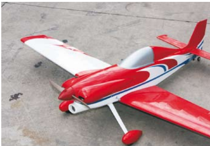
Aerofoil section on this Barbara Jean ARF make this dog of a model suitable for recovering from tip stall practice
