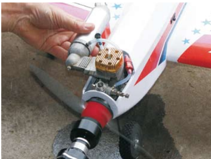
Remove the plug fill the cylinder with fuel and spin it over. Be careful, if it makes your eyes water that's bad. Wear glasses.
