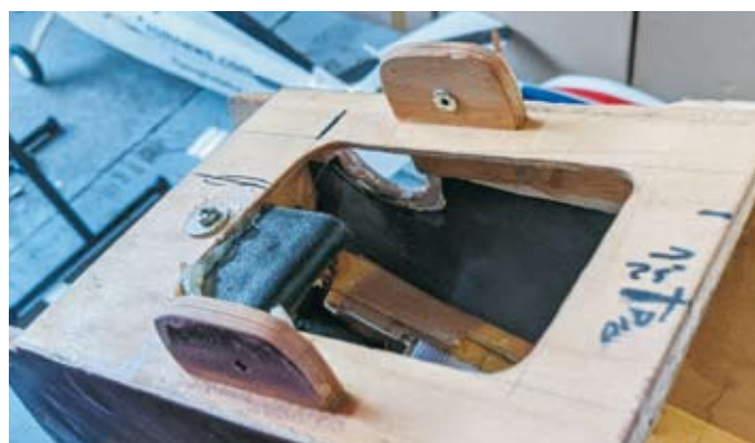
Ballast added fore and aft to meet the now defunct Adelaide power loading rules now removed
