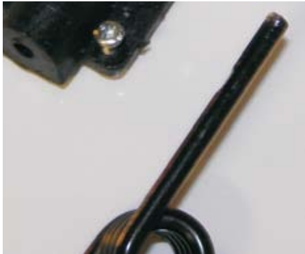
The flat has already been filed on the nose gear steering arm . Do yourself a favour, file one for each the wheel collars as well !
