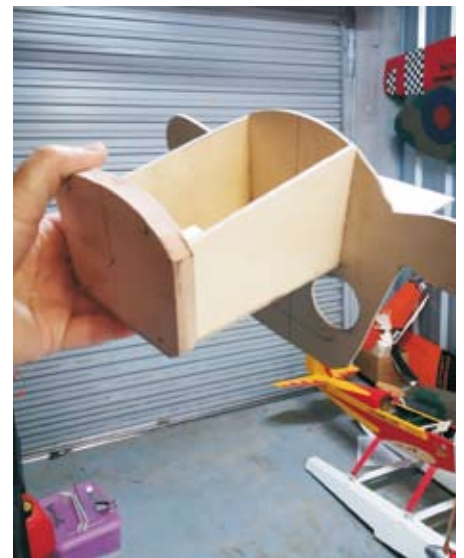
Solid half inch fire-wall for the big bangar
