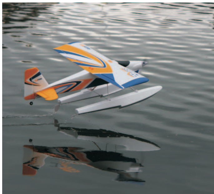
Holding off the conventional way is not the best way to land. Better to fly it on flat with power and skim it on
