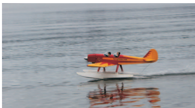
Slight nose up attitude when planing - the Spacewalker is rigged correctly
