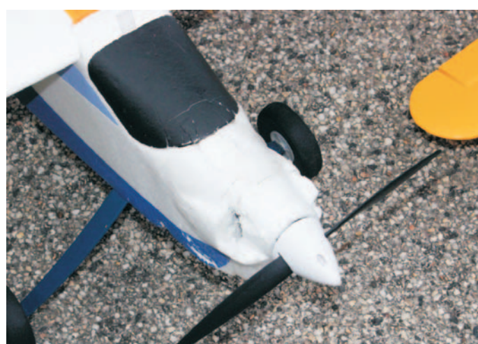
Change the propeller to an 8"x4"
