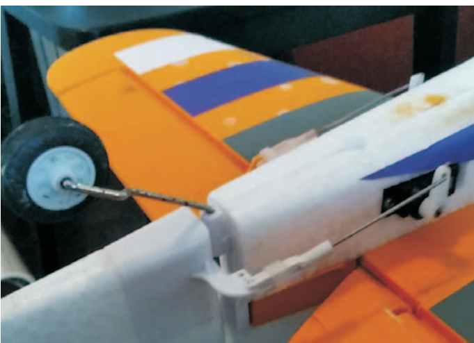
Linkage setup moves Rudder 20mm each way
