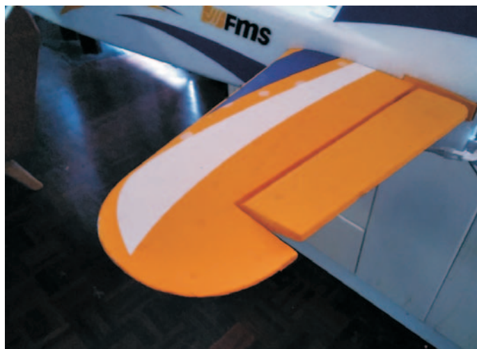
Measured at the trailing edge the Elevator moves up 9 mm
