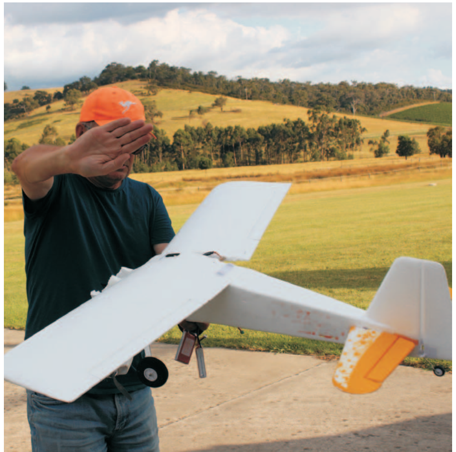
Still flying after a simple patch up with cyano and icy pole sticks
