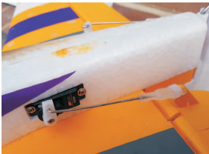
Move Elevator linkage to the second hole out from the centre
