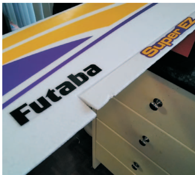
Measured at the trailing edge the Aileron moves up 10 mm
